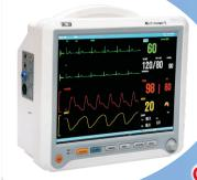
"ECG, NIBP, SpO2, RESP, TEMP, 12.1"" COLOR LED Screen. Built in rechargeable Battery upto 5 Hours working time. 96 Hours Trend graphic data. 90 minutes replaying of ECG waveform. LAN connection. Optional IBP / EtCO2 / Recorder. The user can choose various types of display screen according to different environment like big font display.
